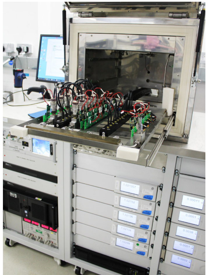
Picture 3: A typical Automated Production Test System
