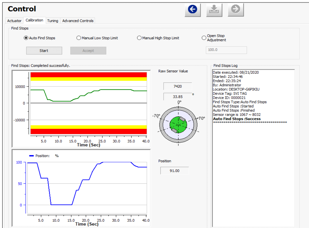
Figure 52 Advanced Setup: Control: Calibration
