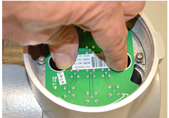
Figure 20: Replacing the board
