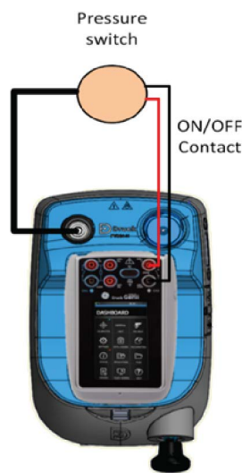
Figure 4-1: Switch testing setup
