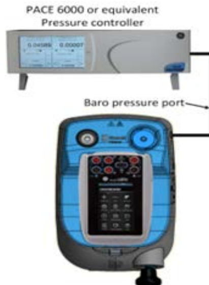
Figure 4-4: Barometer calibration setup
