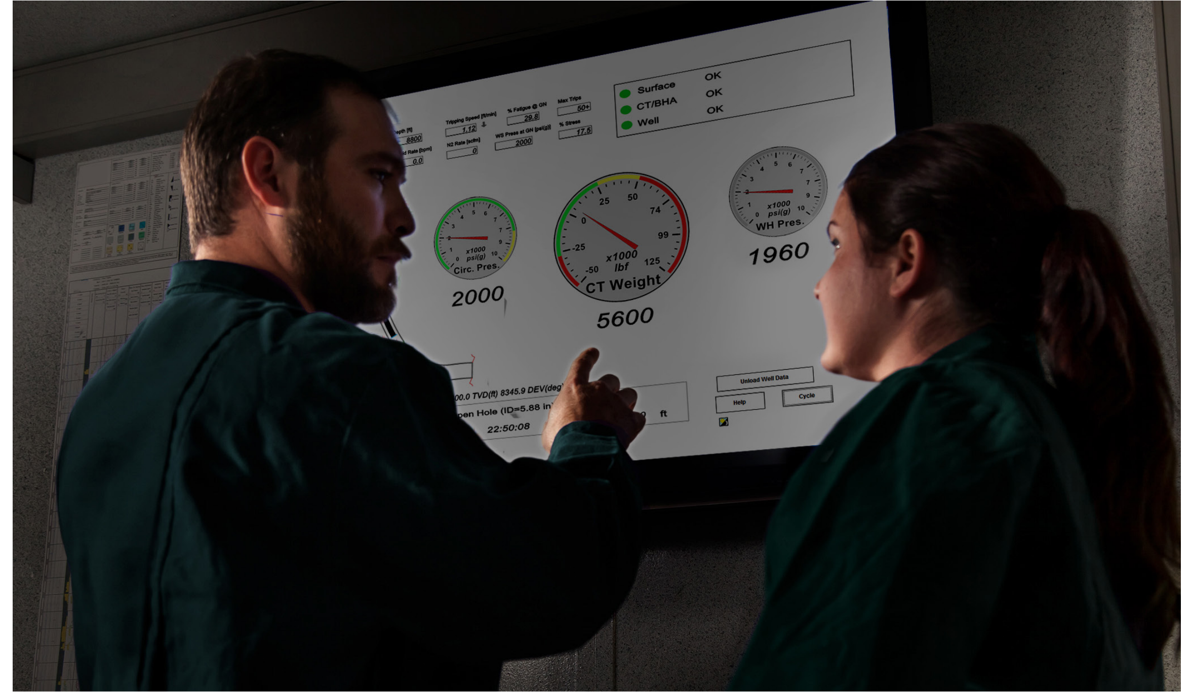
The SureVIEW TeleCoil service retains the use of existing tension/compression/torque (TCT) sensors, effectively supplying a downhole weight gauge to improve service delivery and reduce the risk of tool overload. The TCT sensor data is then added to CIRCA real-time and provides an additional control channel to stop pipe movement via the intelligent injector control system.
