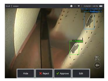
Now save image containing inferences or alternatively cycle through the bounding boxes to 'accept', 'reject' and alter add classification(s) as desired.
