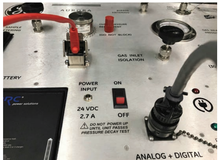
Figure 3: Aurora TransPort I/O cable connections
