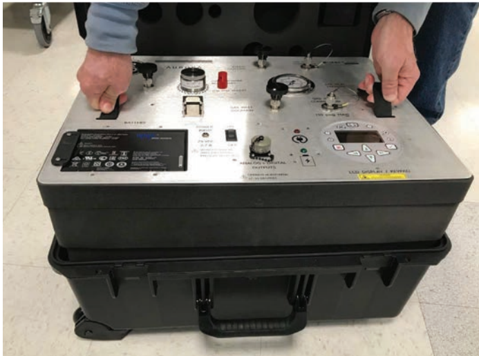
Figure 60: Replacing inner foam housing into the External Pelican case after mirror cleaning
