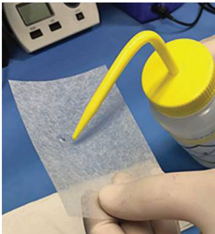
Figure 56: Applying acetone to lens tissue
