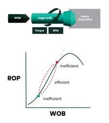
Critical to optimized and efficient milling of wellbore completion components is the ability to provide the required milling parameters of torque, weight on bit (WOB) and RPM, combined with a specifically designed mill bit, in turn delivering optimized rate of penetration (ROP) throughout the task at hand.
